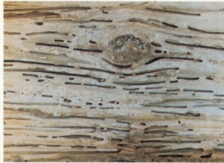
6 — Surface of wood removed to show damage done by termites and the specks of excrement on the gallery walls.
