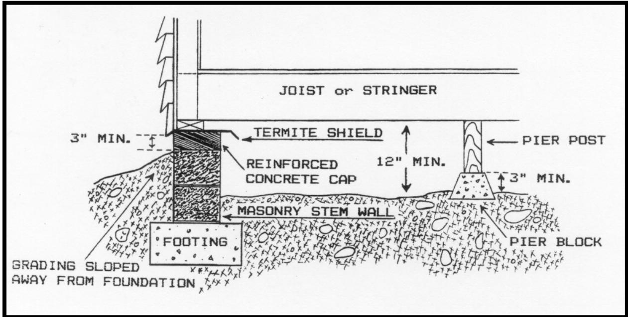
**Figure 1.** Earth to wood contacts and faulty grading are avoided when the location of the wooden members are no less than these indicated and the grading provides adequate drainage. Reinforced concrete caps and termite shields (when properly installed) help prevent termite attack.
