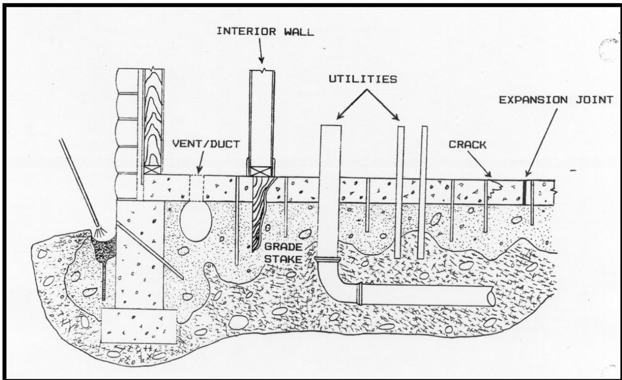
**Figure 3.** Sub slab injection techniques should be used around all utility entrances, expansion joints, cracks and any interior walls which could hide cracks or grade stakes. Slab footings can be drilled at 45 degree angles to minimize and damage or contamination of utilities or duct systems.
