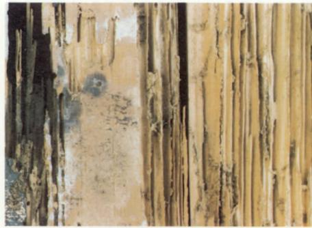
7 — Wood attacked by subterranean termites has a honeycombed appearance because the workers tunnel along the softer grain of the wood.
